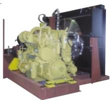
A compact Rig Mount configuration for builders of water well drilling rigs. The 2 stage air end can be provided with Caterpillar engine and side mounted cooler matrix to produce the same air outputs in a base mounted form measuring only 2.25m. x 5.91m. x 2.34m high.
